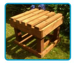
Cut four more 18" frame pieces and screw in at the bottom of the legs.
