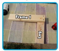
Cut four 13" pieces for the legs, and four 18" pieces for the frame. Screw each frame piece to each leg at a right angle as shown.
