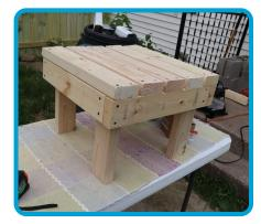
Measure across the frame from outside to outside (in this case it was 19.5"). Cut five boards and screw into the top of the frame.
